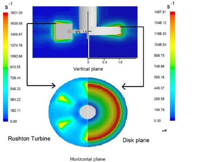
Figure 1. Shear rate at the same power draw ( $P=12.92 \text{ W}$ )
